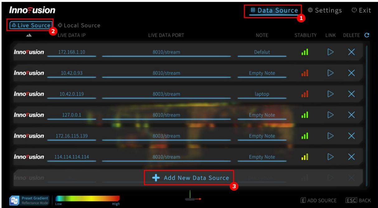
3. Enter LiDAR IP address and port number. Click
