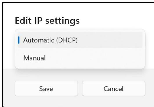
5. Toggle on **IPv4**. Enter the **IP address**, **Subnet mask** and **Gateway** to make the computer with the same subnet to the LiDAR. See below for example of the settings for a default factory LiDAR. Click **Save** to save the settings.
